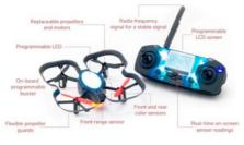
ACCELEROMETER FOR SENSING ACCELERATION GYROSCOPE FOR SENSING ROTATION BAROMETER FOR SENSING HEIGHT AND PRESSURE FRONT RANGE FOR SENSING OBSTACLES AHEAD **BOTTOM RANGE** FOR SENSING DISTANCE TO THE GROUND COLOR FOR SENSING SURFACE COLORS **OPTICAL FLOW** FOR SENSING RELATIVE POSITION
